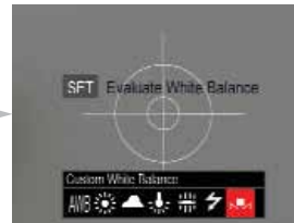
Zoom in so the EzyBalance fills the whole frame of the camera and take a reading off the card (refer to your camera manual for instructions).
